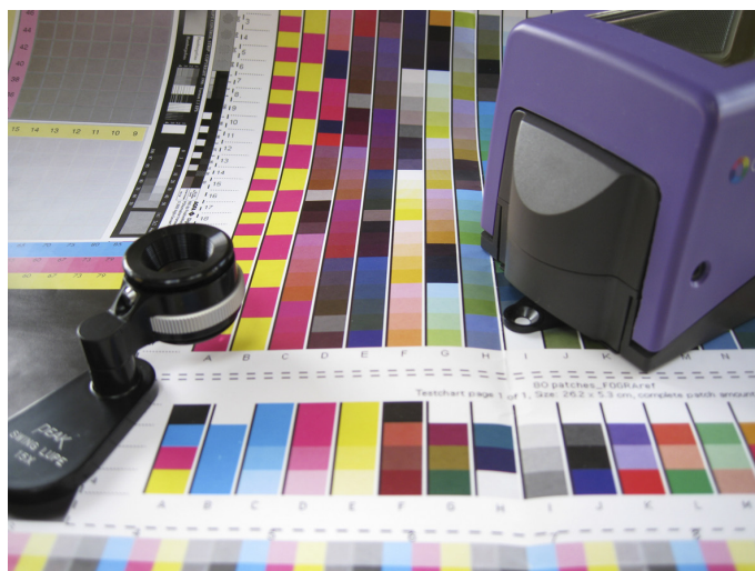
One of the most important measuring devices in print production is the spectrophotometer. This should be serviced and calibrated regularly by an ISO 17025 accredited laboratory.
