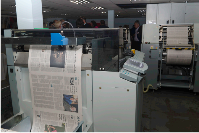
This shows a newspaper going through a Hunkeler finishing line at Stroma, having just come off an Océ Jetstream inkjet printer, which is in the background.
