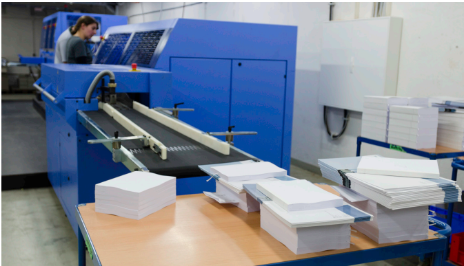
Books are lined up ready to go into the Diamant MC Hybrid bookline, separated into batches according to their thickness.
