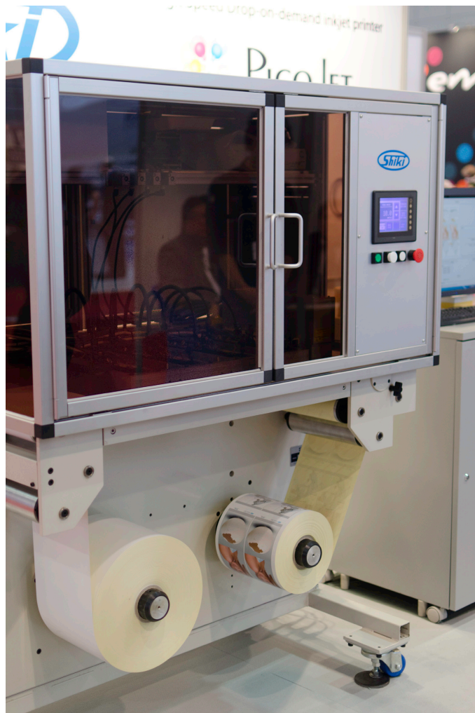
Japanese firm Shiki showed off this prototype inkjet printer which boasts an impressive 50mpm despite its relatively small size.
