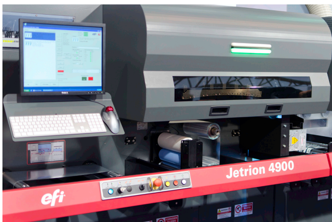
EFI has added inline laser die cutting to its Jetrion inkjet press with the launch of this 4900 model
