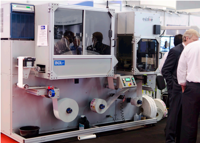
Spartanics demonstrated this digital label printer, based around Xaar 1001 heads and which incorporates laser die cutting.
