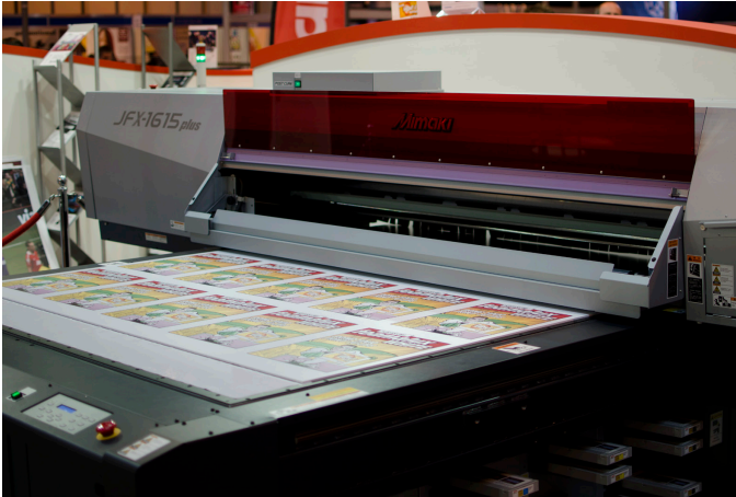
Mimaki demonstrated its new JFX-1615plus, a flatbed UV printer with LED curing.
