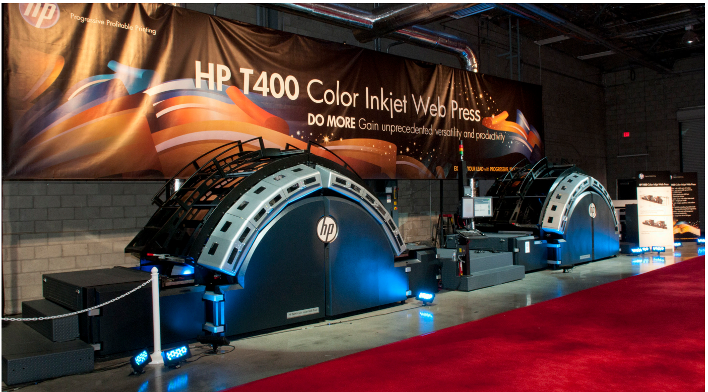
HP's latest addition to its Inkjet Web series is the T400, a 42-ins printer capable of a production speed of 183mpm.
