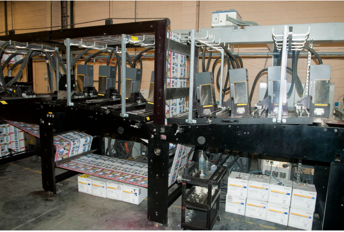
Lettershop had this tower purpose made to support its eight S10 heads plus four of Kodak's older 91 series heads for black printing.
