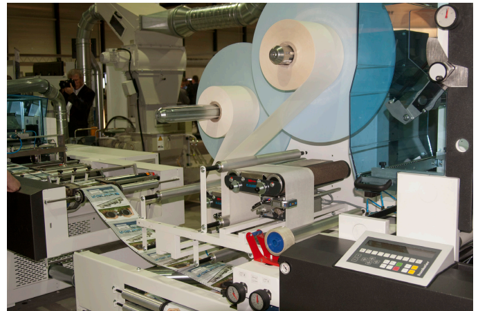
Hunkeler's Double Plow fold unit as demonstrated with its book production line.
