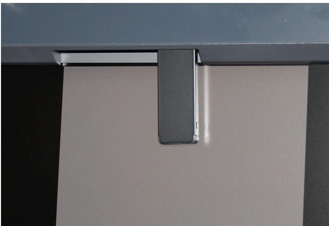
The built-in measuring device is a colorimeter that swings into place when the operator pushes the "Calibrate" button, or calls for a re-calibration from the software provided with the monitor.
