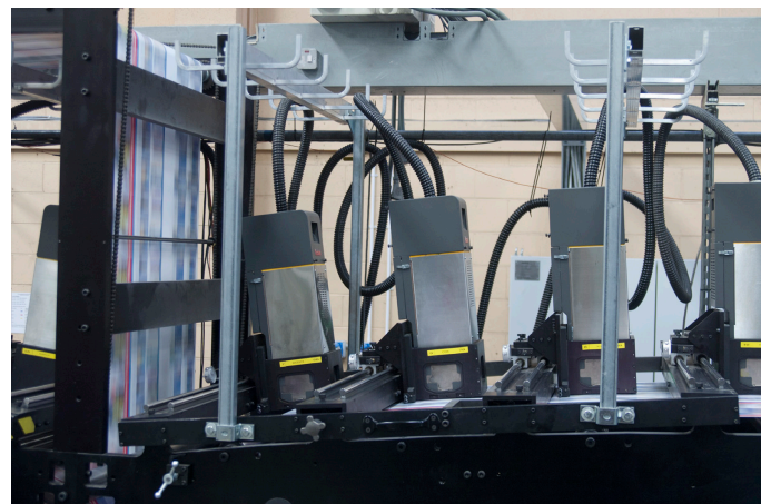
These Kodak Prosper S10 heads produce 600x600dpi resolution and a 175 screen ruling.
