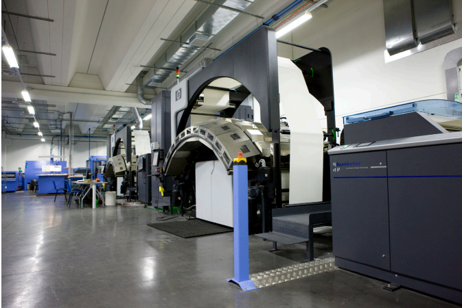
The HP T300's curved paper path optimises ink/substrate performance.
