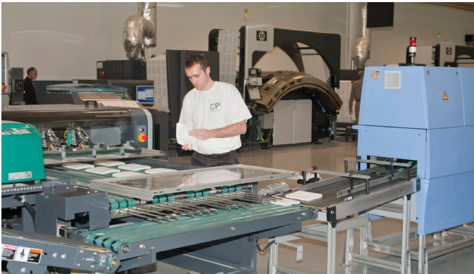
CPI's plans for the T300 revolve around the Quantum production line which converts the printed web into bound book blocks.
