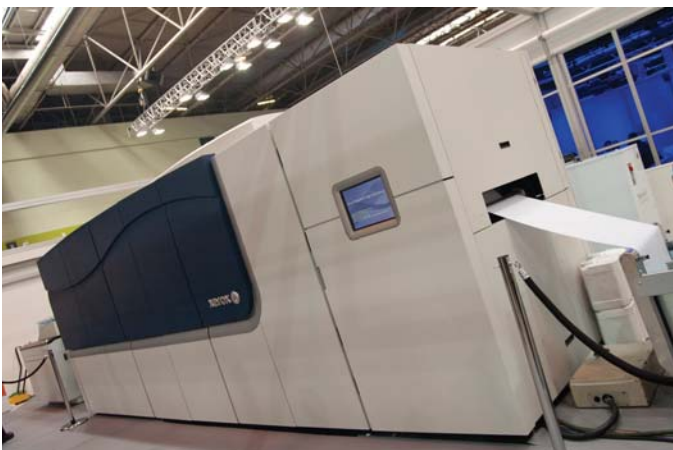
Xerox's Production Inkjet printer is designed specifically to print to lower cost media, targeting the transactional/ transpromo markets.
