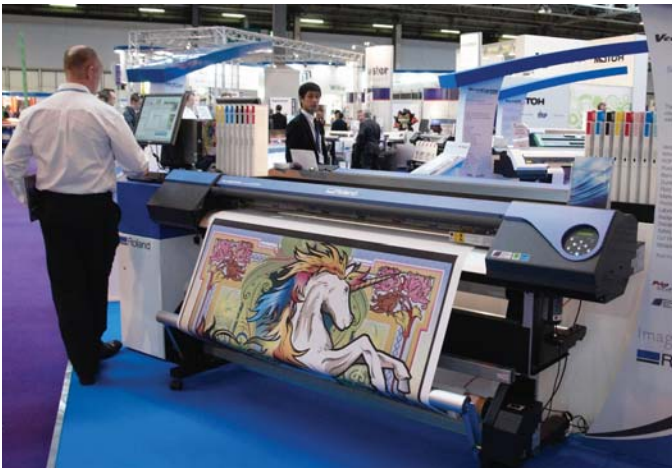
Roland's VersaCAMM VS-640 solvent printer allows metallic silver to be mixed with process colours for novel effects.
