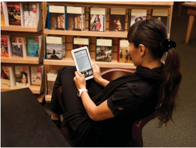
Barnes & Noble's Nook uses two screens: a monochrome one for the e-books and a colour one for the user interface.
