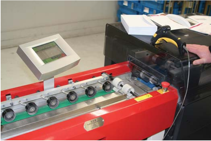
The Strålfors Reliable Mailing system, SRM, includes both hardware development (readers of Data Matrix 2D barcodes) and software to keep track of print and rejects in the workflow.
