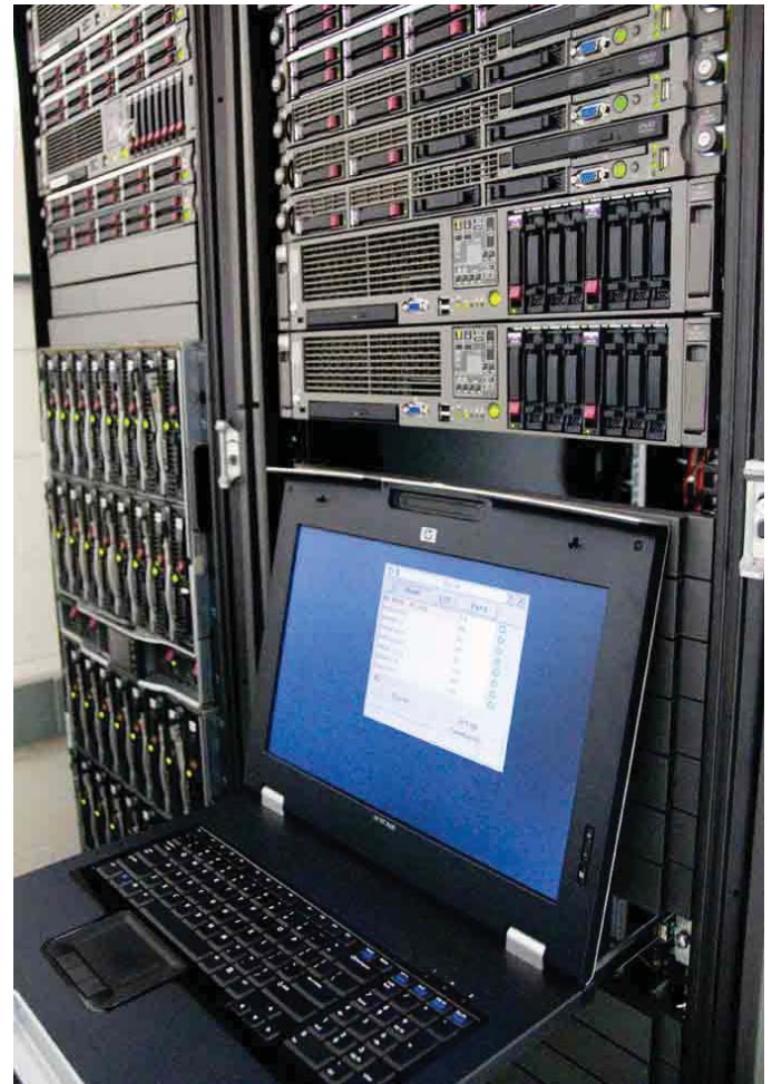
The SmartStream Ultra DFE has an astounding 144 Harlequin RIPs, mounted three per blade on 48 multicore blade servers.
