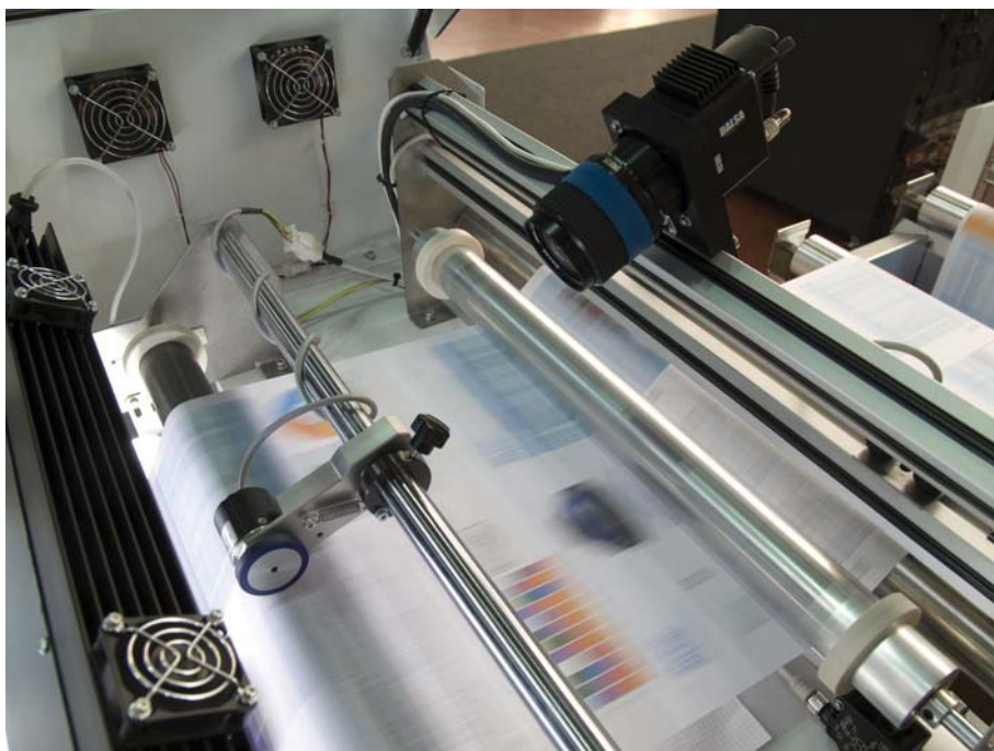
The Web Inspection module is a high resolution camera that can verify that the right elements have been printed.
