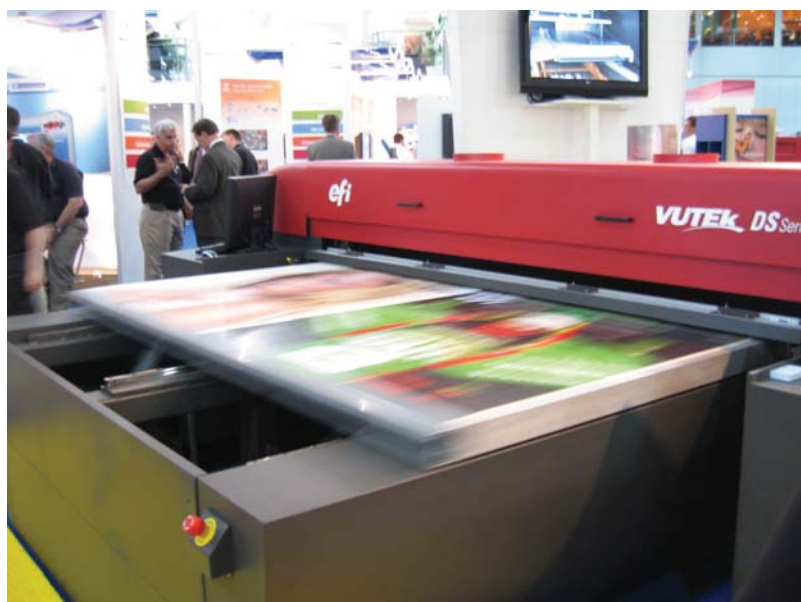
EFI has shown off this Vutek DS8300 which claims a top speed of 557sqm/hr.
