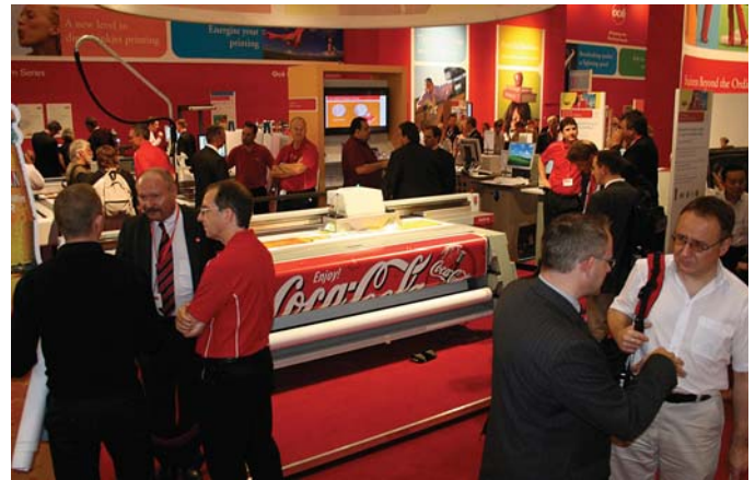
The Océ Arizona GT combines flatbed design with roll-to-roll capacity. It uses UV curable ink and variable ink drop size from 6 to 42 picoliters.
