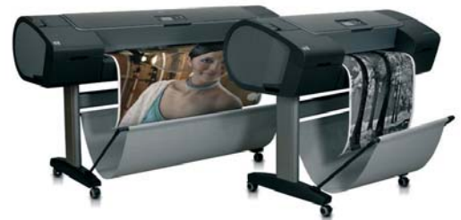
The HP DesignJet Z3100 was the printer that could reproduce the purple spot colour closest to the real print. This is because it's a twelve colour printer using CMYK plus light magenta, light cyan, red, green, blue and two different blacks and greys, plus gloss enhancer.
