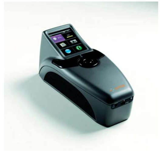
To measure CTP-plates you need a dotmeter. Here the Plate Scope from X-Rite, which can read low contrast plates as well as different screen types.
