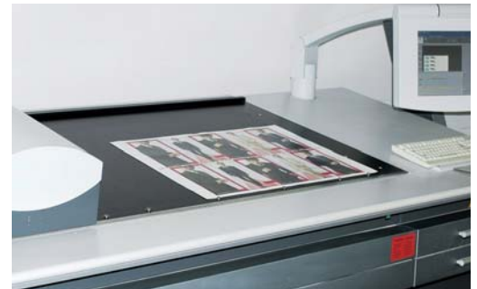
While densitometers still have their place in print production, you need a spectrophotometer to measure the true colours. Pictured is Heidelberg's Princt ImageControl.
