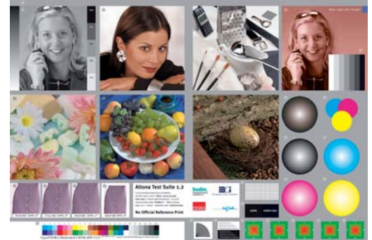
One of the test forms, used before by us when testing digital printers and proofers, is a page from the ECI Altona Test Suite. It contains several types of images to evaluate visually, as well as a control strip for spectral measurements.
