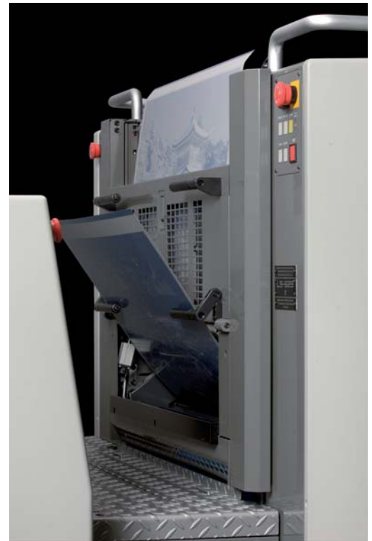
Automatic plate changing technology on Komori's B2 Lithrone S40SP Series can change plates on a ten unit press in a only five minutes.
