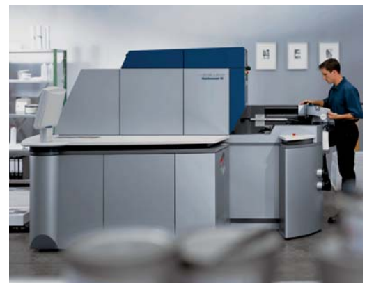
Quickmaster 46 DI from Heidelberg has built in ctp, one imaging unit per plate cylinder. It's a two-up printing press (34 x 46 centimeter sheets).
