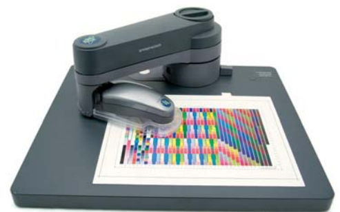
The Gretag-Macbeth robotic measuring device Eye-One iO reads a typical test chart in less than two minutes. This device was used for the tests (see page 28).
