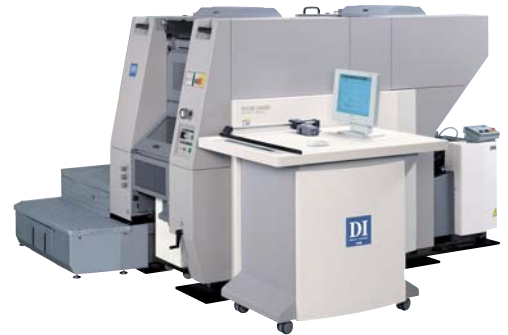
The Ryobi 3404 DI is designed in close cooperation between Presstek and Ryobi. The design is clearly inspired by 74 Karat, but this is a two-up press (34 x 46 centimeter sheets).
