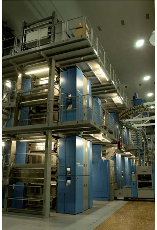
Among the newcomers in DI-imaging is the Swiss newspaper press manufacturer Wifag. The Evolution DI web offset press has direct imaging of the plates, on press. The first installations are at present run in test production.
