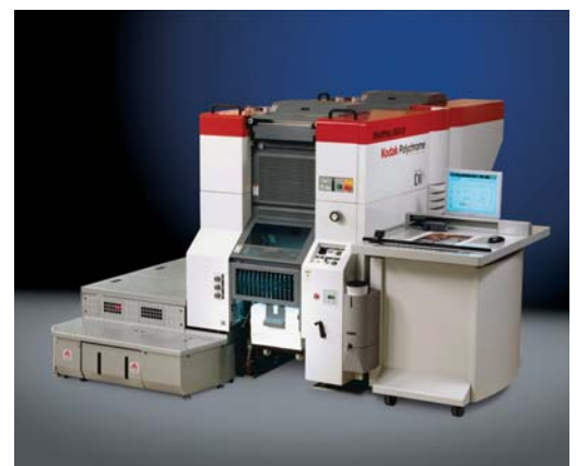
The Kodak Direct Press 5634 is yet another DI-press based on the Ryobi 3404. For Kodak it is a complementary product to the other digital presses in the portfolio, the Nexpress and the Versamark.
