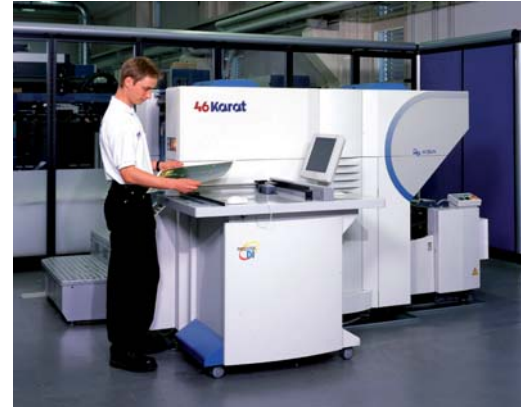
The 46 Karat from KBA is just like the "bigger brother" 74 Karat using waterless printing technology. It's actually manufactured under license by Ryobi for KBA.
