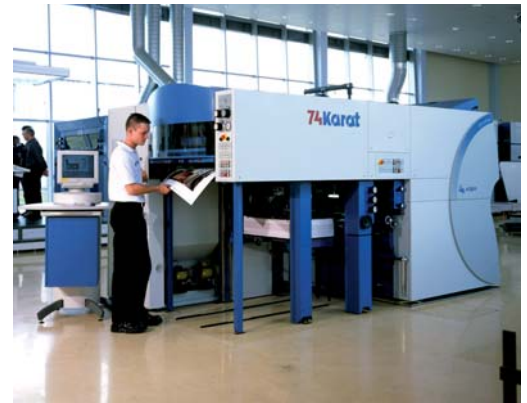
The 74 Karat from KBA uses waterless printing technology and is a four-up press (52 x 74 centimeter sheets). Some use it as a proofer for longer print runs.
