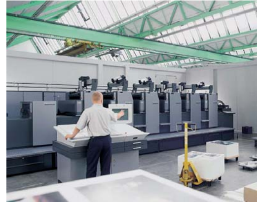
The Speedmaster 74 DI from Heidelberg can be extended to up to six printing units, all with built in CTP. Pictured is a four-up printing press (53 x 74 centimeter sheets).
