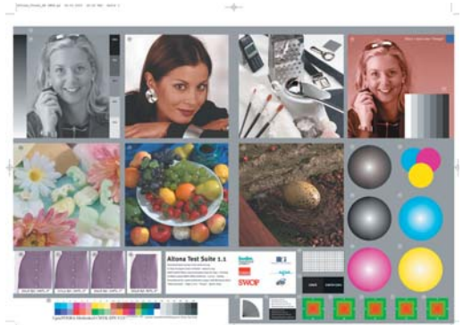
(Figure 1) The test page called Visual has a lot of different images to help evaluate different aspects of imaging quality.
