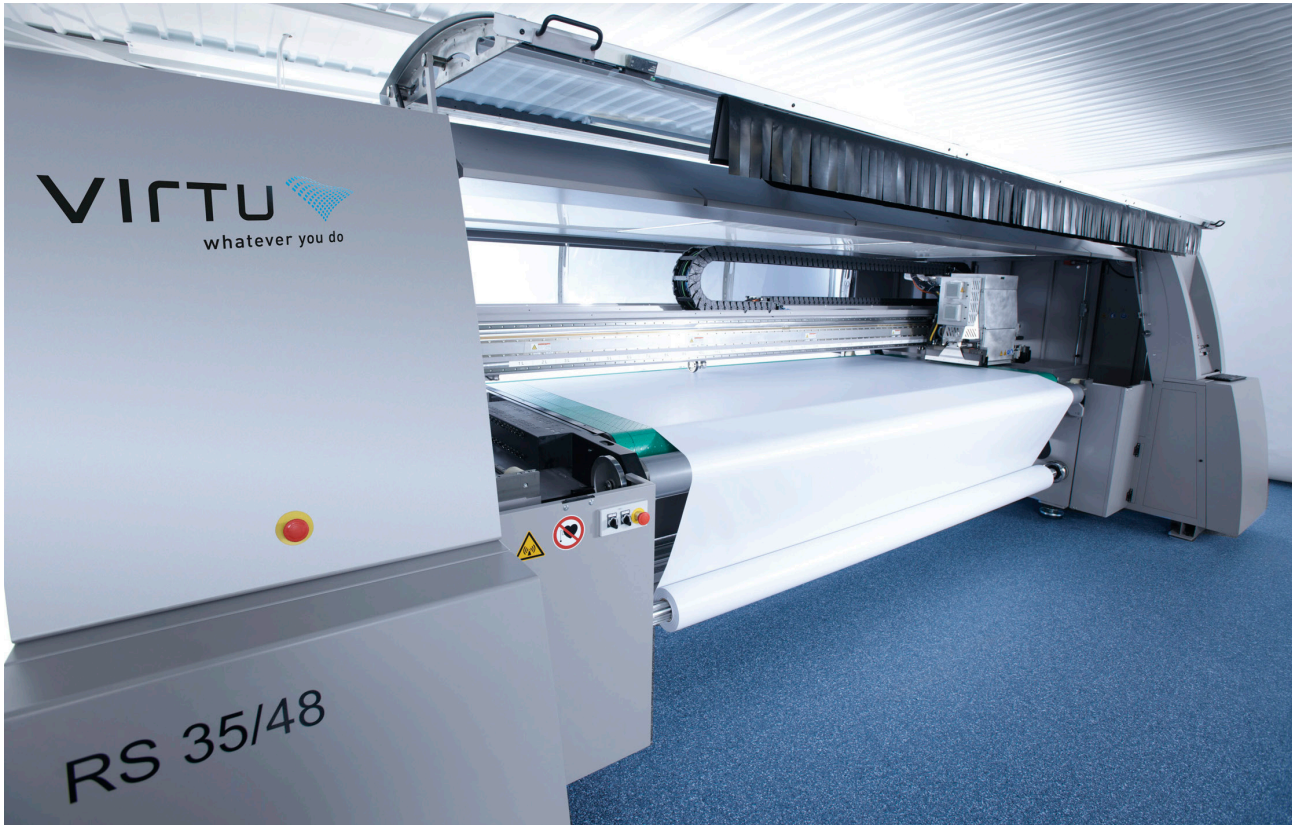
The Polytype SA Virtu RS35 is a hybrid UV-printer able to print up to 3.5 m wide media, and up to 95 mm thickness.
