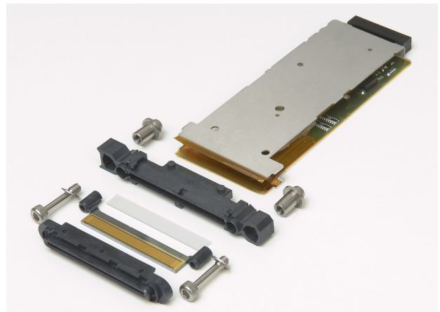
HP Scitex's X2 print head is designed for extremely high throughputs. It can be assembled into multiple head modules for output resolutions of up to 800dpi, according to HP.
