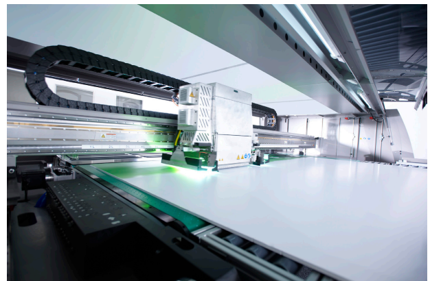
The vacuums in flatbeds must be strong enough for heavyweight substrates. Here the Polytype Virtu RS35.
