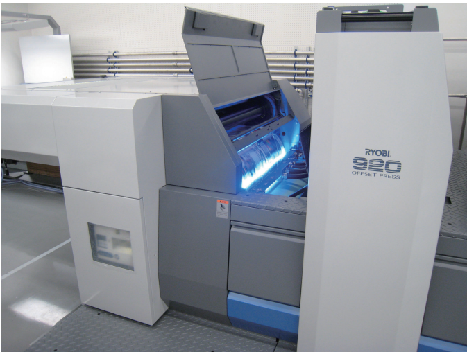
Ryobi was the first press manufacturer to introduce LED UV curing, seen here on a Ryobi 920 press.
