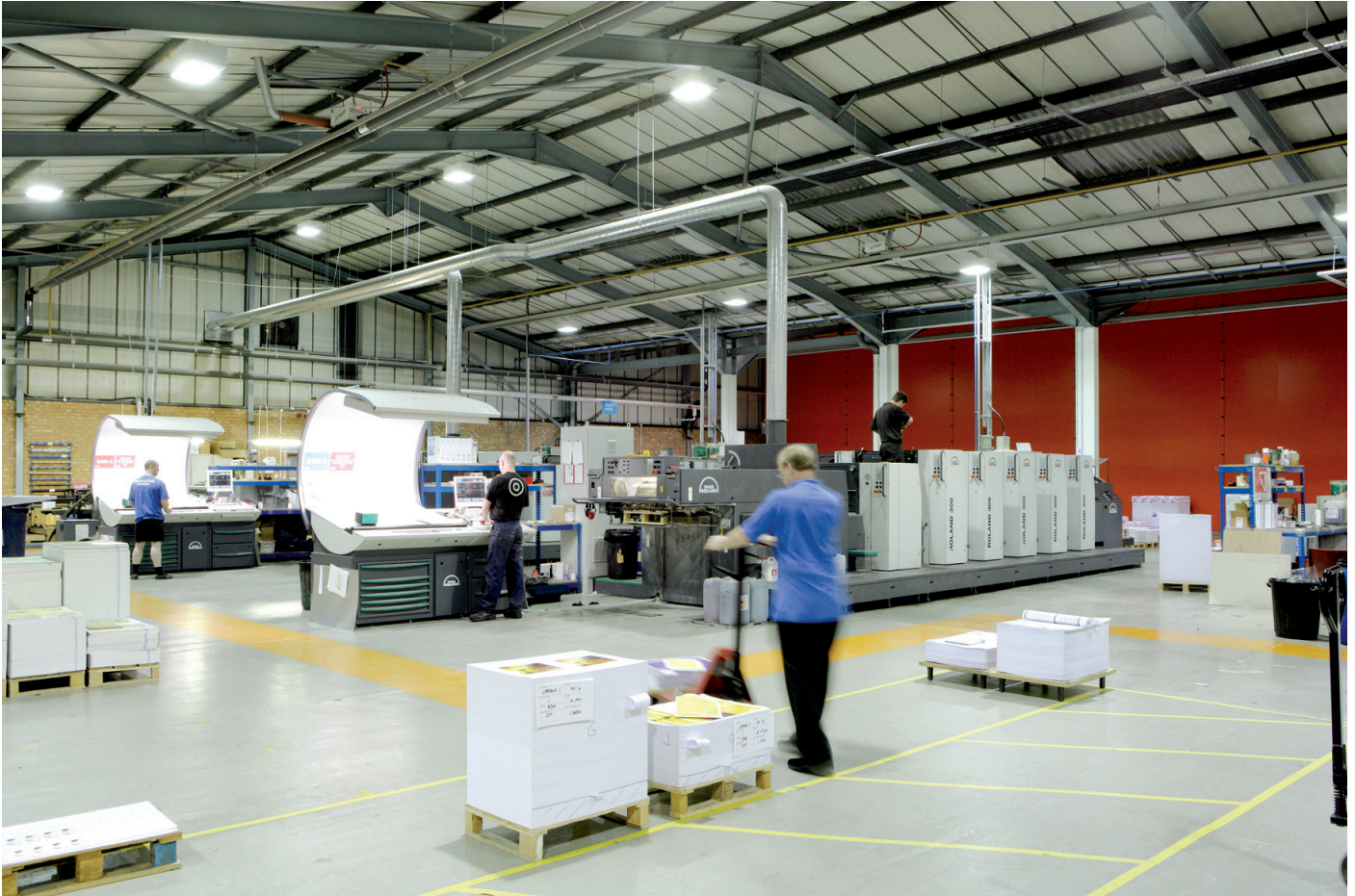
The company has both digital and conventional presses. This ManRoland 500 can print 18,000 sheets per hour. Look at the speed that man's moving to feed it!
