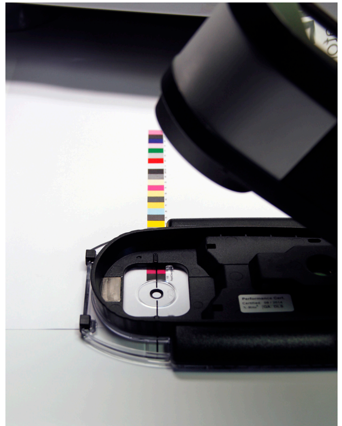
The X-Rite eXact spectrophotometer can now be used in scan mode, measuring one or several rows of a control strip in a fast and efficient way.
