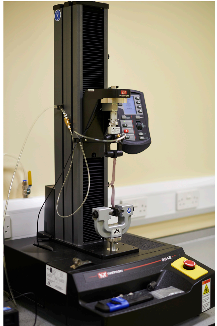
To test how customer inks might react with the adhesives used in the construction of the printheads, this device pulls the layers apart, while measuring the amount of force needed. Photo © Nessian Cleary
