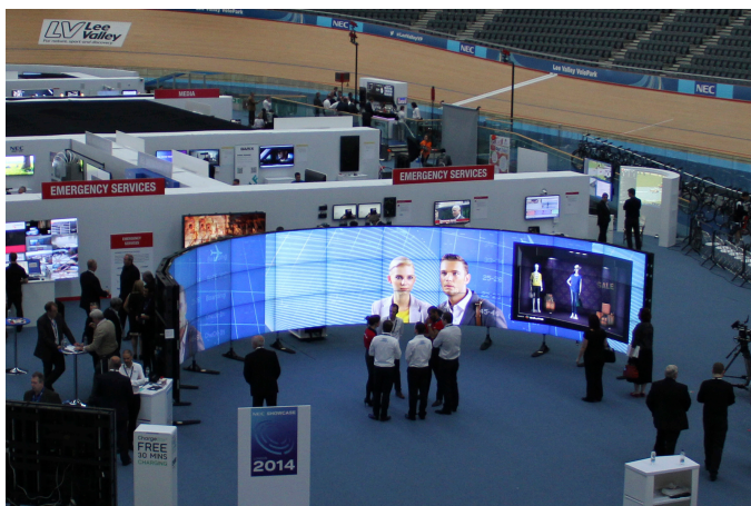
The UK vendor PSCo created a 180-degree curved display using in all 36 individual 55-inch NEC panels at the NEC Showcase.
