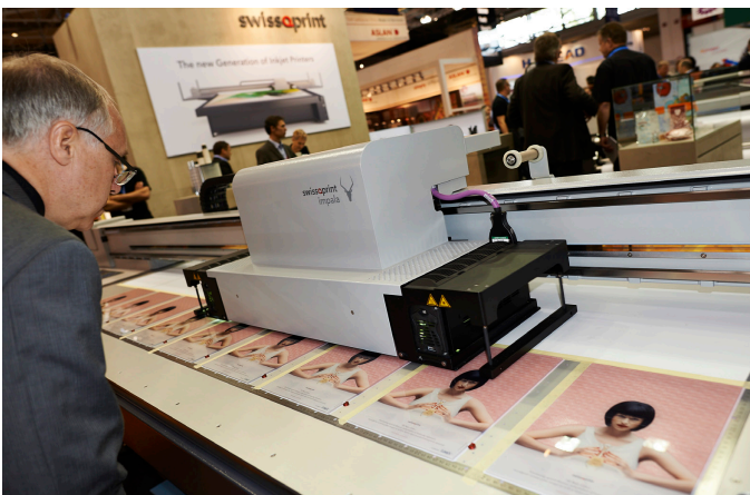
SwissQPrint demonstrated an Impala UV flatbed printing an effective lenticular that can be applied to any part of an image.
