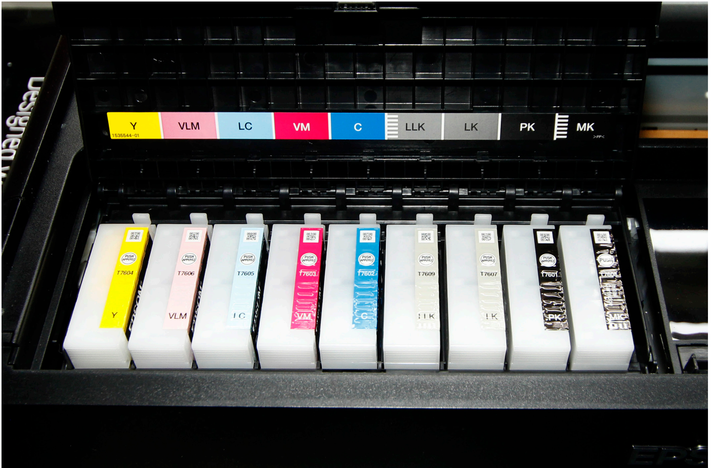
The SureColor P-600 has in all nine inks, all in separate cartridges. There are two different blacks, and special light grey and mid grey for a smooth rendition of B/W photos.
