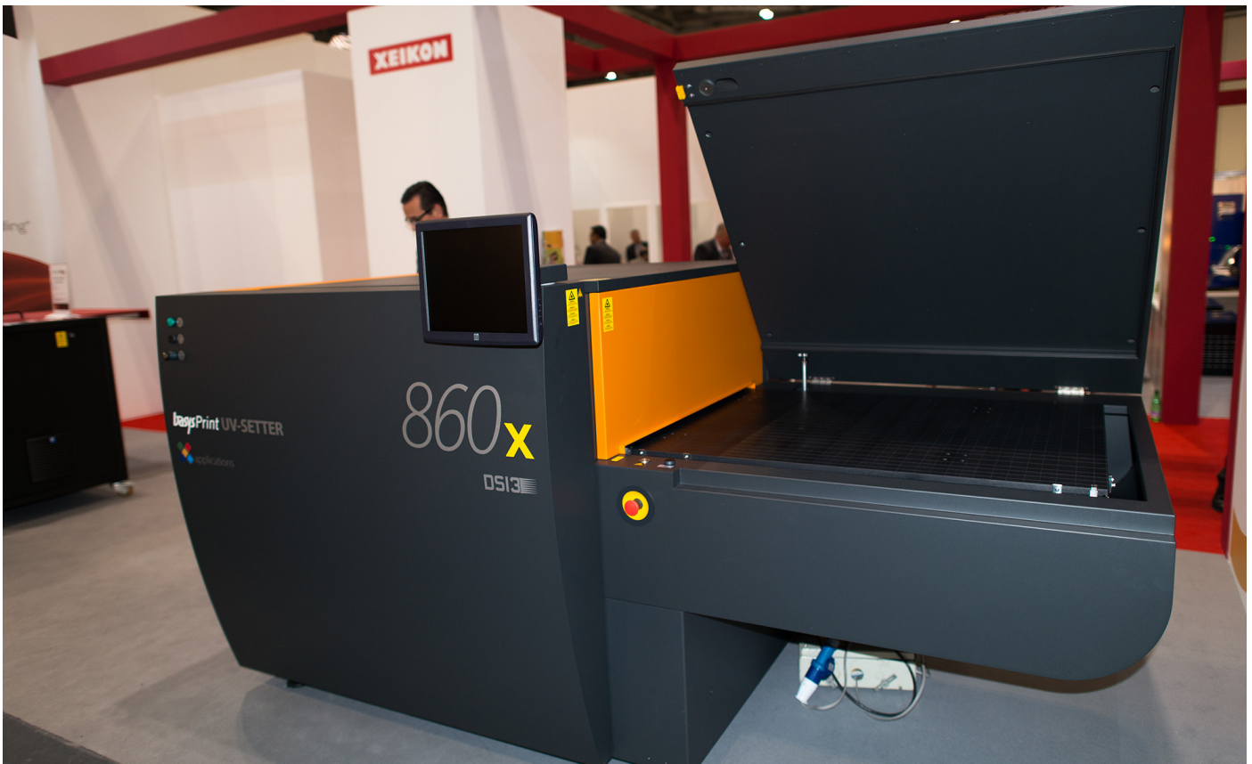
The BasysPrint CtP devices, such as this 860x that was on the stand at IPEX, work with UV sensitive plates.
