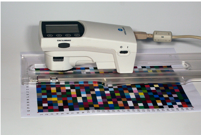
The FD-7 spectrodensitometer from Konica Minolta Sensing supports measurements in ISO 13655 M1-mode, as well as scan mode and measurements of ambient light.
