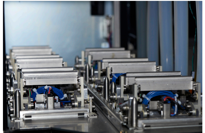
At the heart of the system are these Kodak print heads, identical to those fitted to the Prosper presses.
