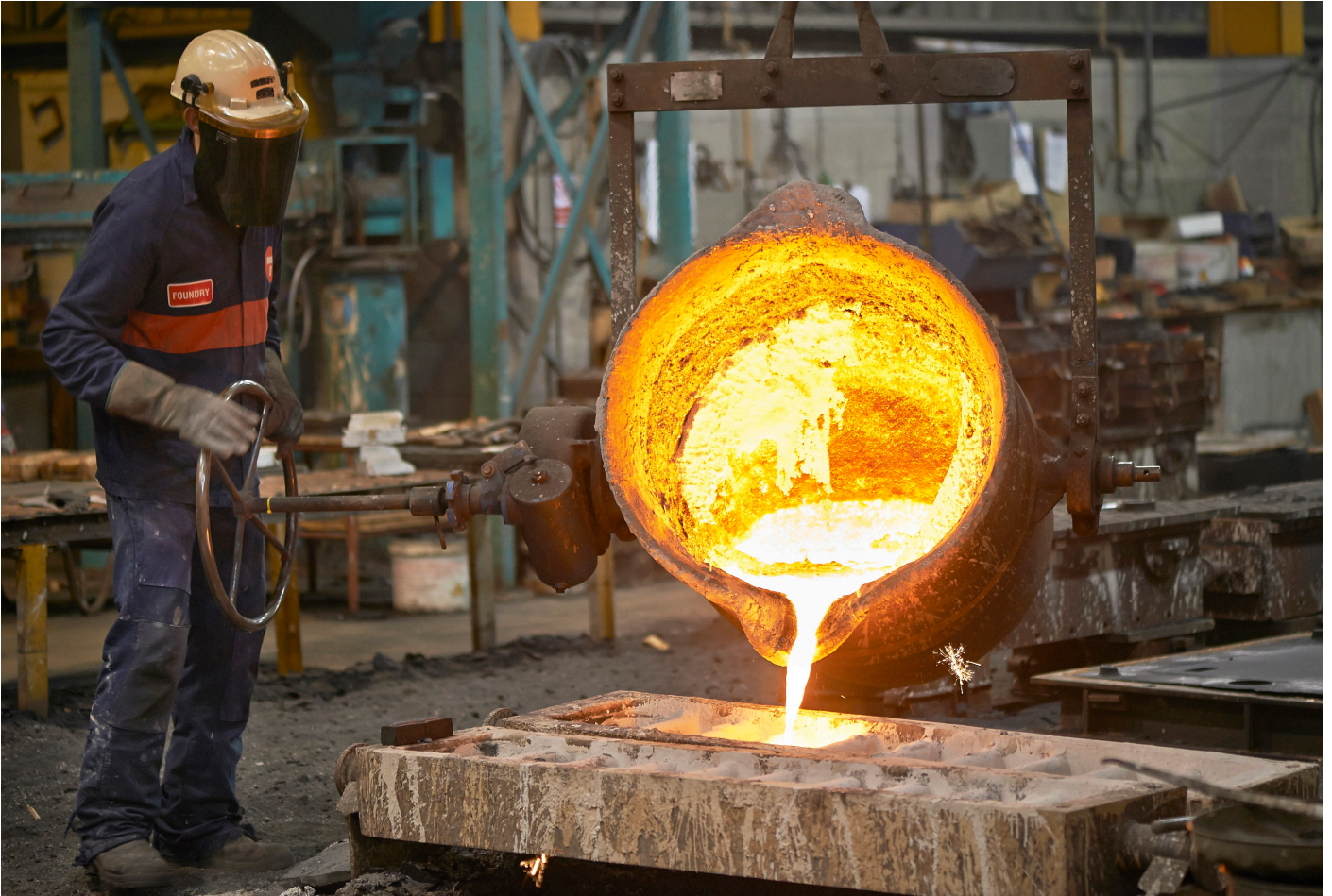
Timsons operates its own foundry - here molten iron is being poured into moulds.
