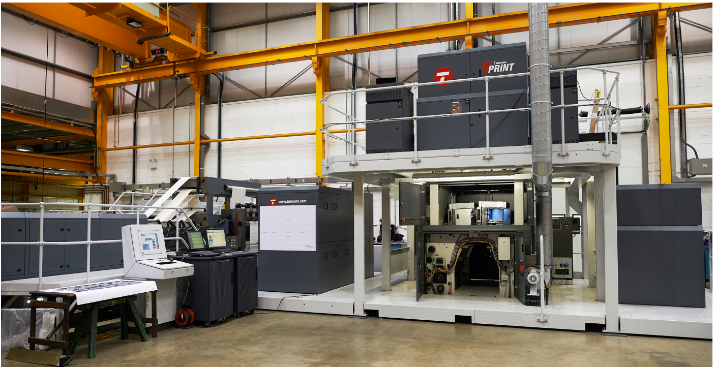
The Timsons T-Print is a large press, with the paper passing through one set of printheads, then folding back on itself to print on the reverse via a second set of printheads in the upper deck.
