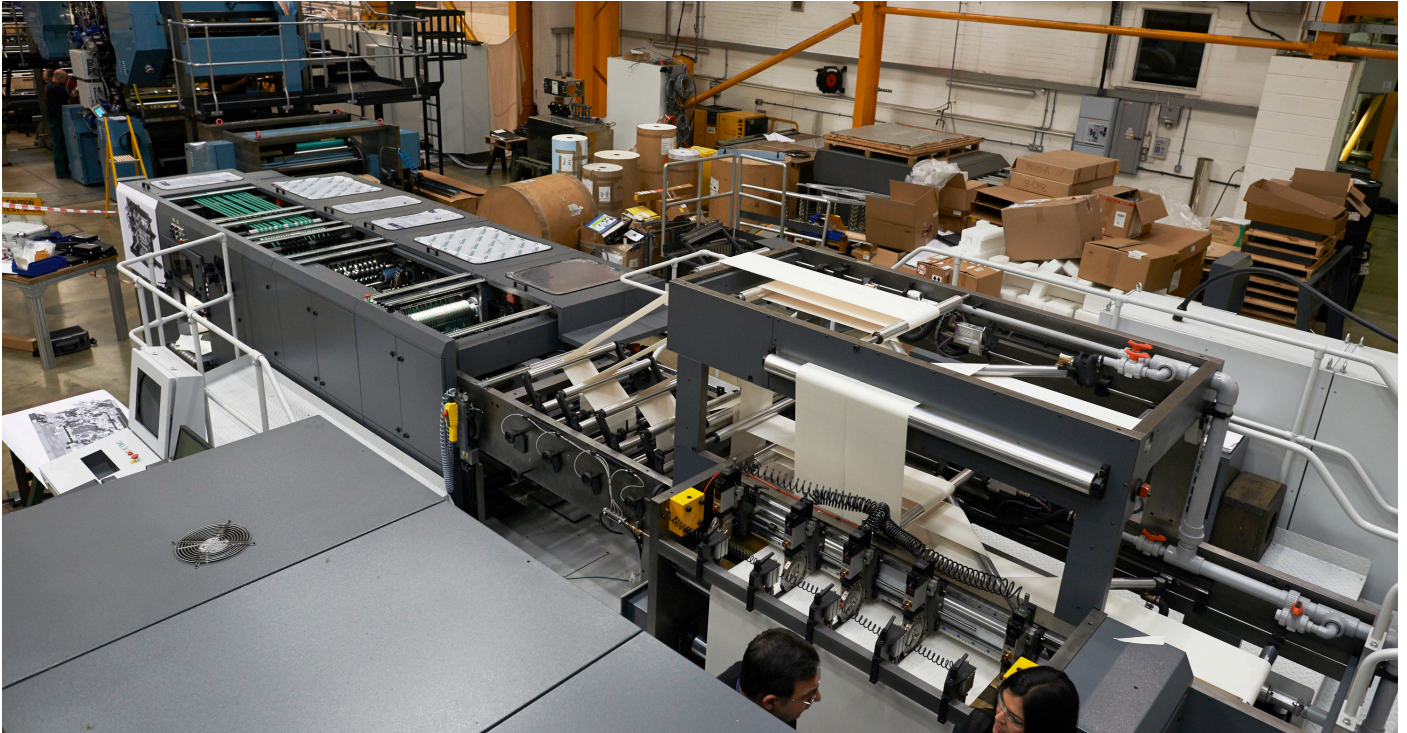
The T-Fold takes the web from the back of the T-Print.
