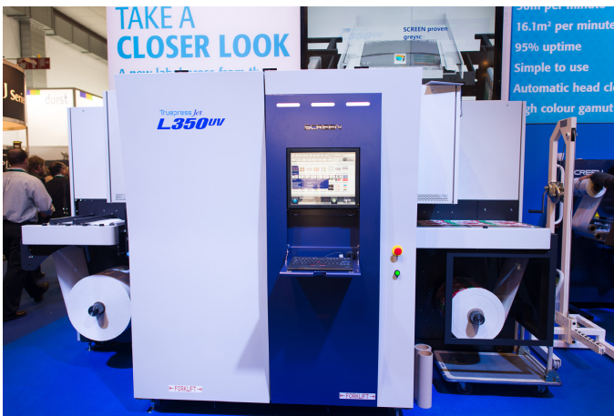
Screen launched its Truepress Jet L350UV, a single pass UV inkjet label printer.
