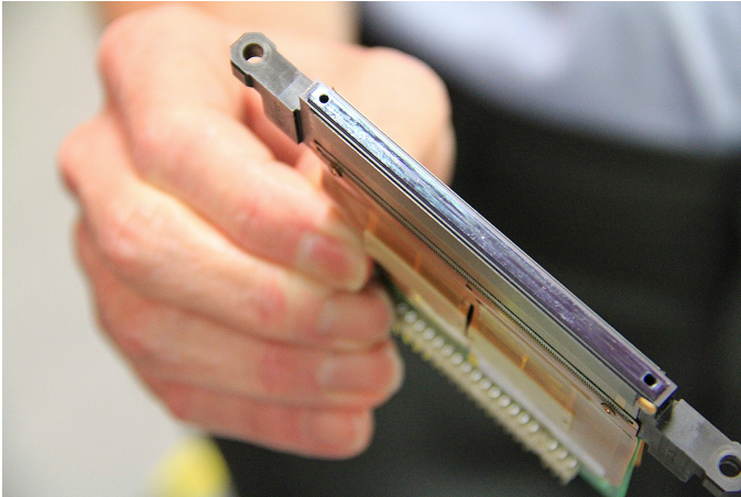
The 256-nozzle Q40i printhead is a hybrid of full MEMS heads that have the silicon nozzle plate, and the older head design used on the S20.
