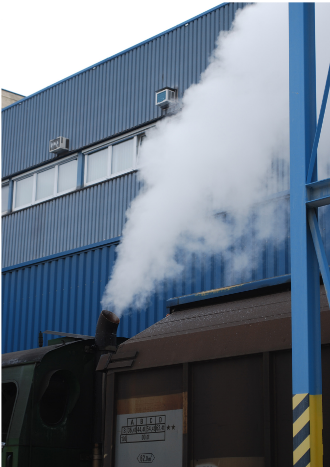
The Mondi Neusiedler mill in Austria uses a steam train to transport incoming pulp to the paper machines a few hundred yards away. The steam is good for about six hours use in the train and is captured as waste from the paper making process.
