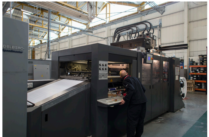
Kodak Prosper print modules fitted to the top of the CutStar unit on a Speedmaster at the Anton Group.
