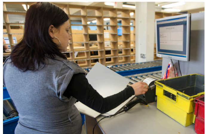
Screens on the shop floor tell operators what process to carry out and for which jobs, while tickets are printed out and added to each batch.
