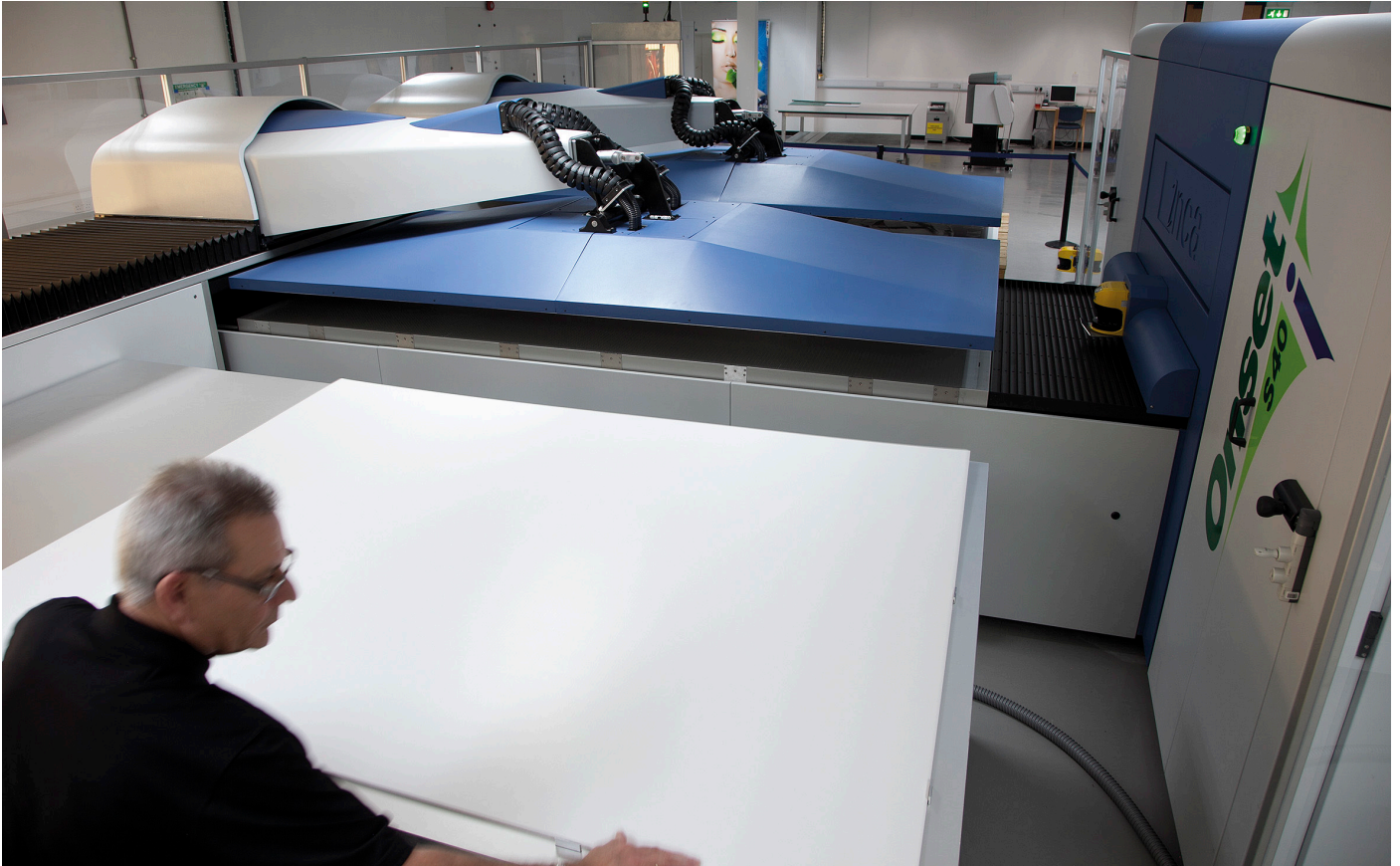
Fujifilm's new corrugated handling system for the Inca Onset S40i.
