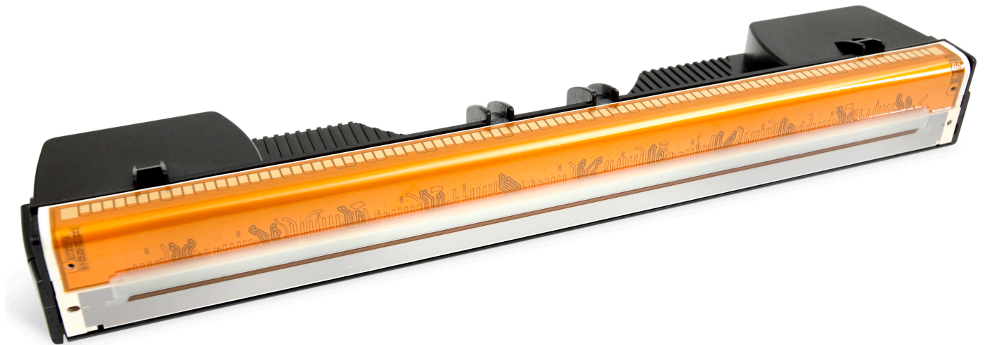
The Memjet printhead is designed as a page wide array, 220mm wide, and containing five ink channels. It's a consumable unit, but it's easy to snap replacement heads in.
