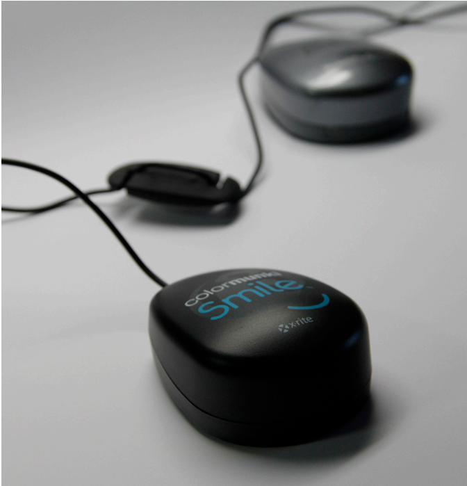
The ColorMunki Smile is a low priced monitor calibrator from X-Rite which looks very much like the older Eye One Display (shown in the background of the picture).
