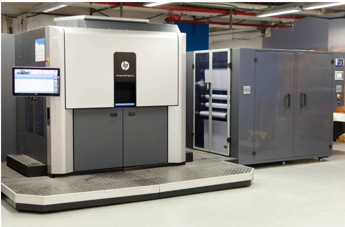
This B2 Indigo 30000, seen here sitting in the Indigo factory in Israel, is designed specifically for folding carton.
