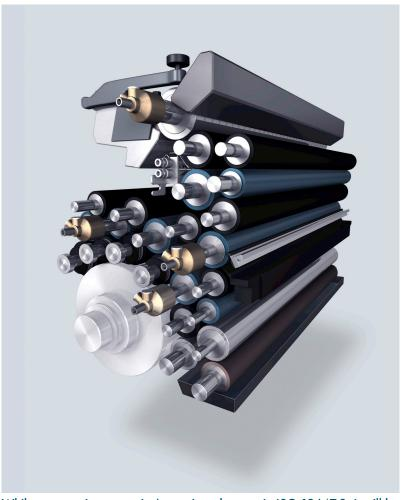
While press maintenance isn't mentioned per se in ISO 12647-2, it will be difficult to stay within tolerances of TVI, colour deviation and variation if the press isn't serviced according to the manufacturers instructions.
