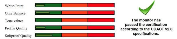
A monitor should be calibrated to the ISO 12646 standard if used for high end soft proofing. Checking the compability of the monitor with this standard can be done using for example UGRA's UDACT software, or other similar monitor validation tools.
