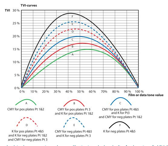
A central task in plate preparation and press calibration is to check and adjust for dot gain, called TVI (Tone Value Increase) in the ISO 12647-2 standard. This will be different for different types of plates, papers, screen types and inks.
