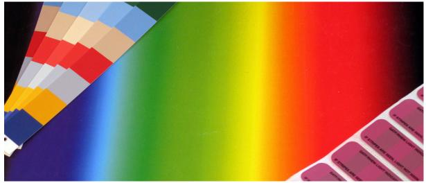
The character of different light sources will effect how the colours are perceived when viewed. A proper viewing booth uses a light source with good spectral distribution of all the wavelengths, and with a white point at 5000 K. A light indicator card like the GATF RHEM card will show banding if the light isn't correct.
