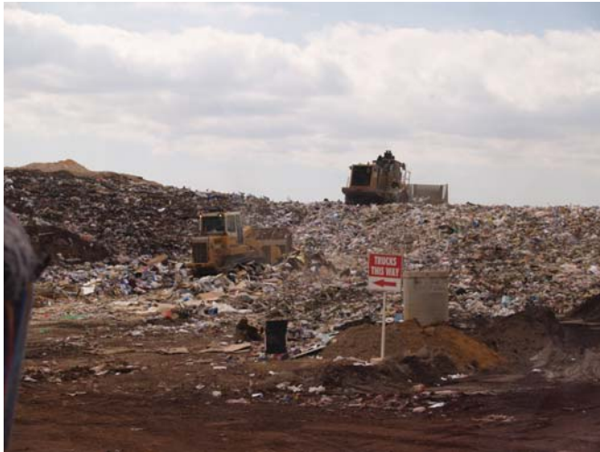
Active tipping area of an operating landfill in Perth, Western Australia.
