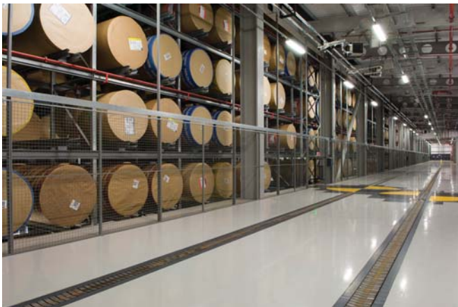
At peak times reels are delivered every 15 minutes with up to one week's worth of paper reels automatically unloaded and moved to store in this high bay.
