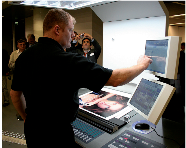
The latest generation of press control systems, like the Komori K-Station (above), can generate or modify ICC profiles based on the actual print run.
