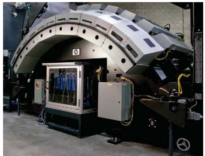
HP's giant Inkjet Web Press uses a bonding agent to help the ink stick to the paper, but this also helps to make it easier to deink for recycling.
