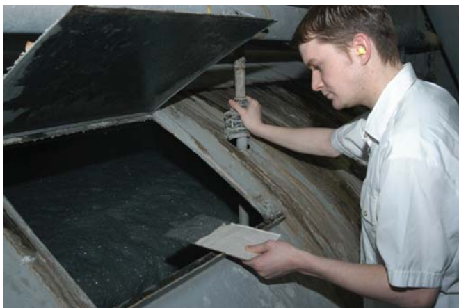
The air bubbles used in the flotation process can clearly be seen here in this image from Aylesford Newsprint.
