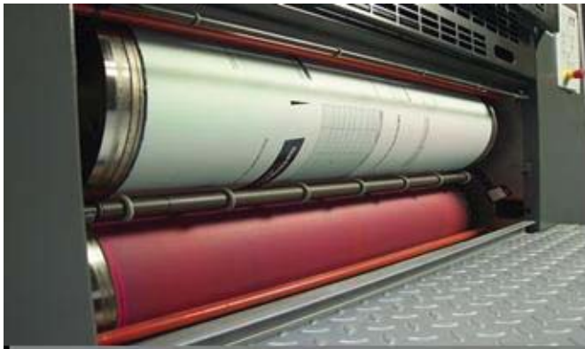
Kodak's Thermal Direct relies on the fount solution to moisten the non-imaged coating, so that the tackiness of the ink pulls the coating off on the first few press sheets.
